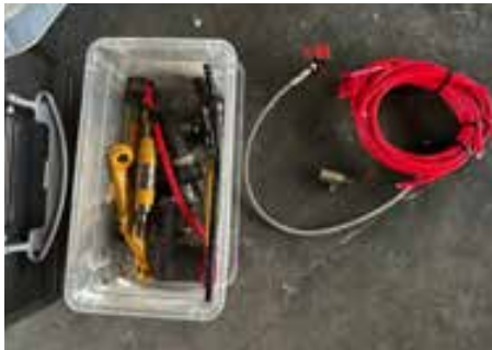
Yellow means crack tested front end components Rocker gear direct oil feed
